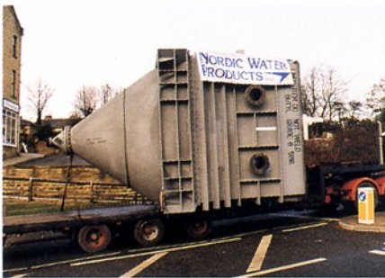
RUBBER-LINED PLATE SEPARATOR DESIGNED FOR DESULPHURISATION PLANT.
